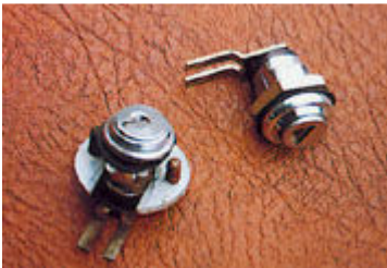
The old original door lock on the left fitted with a modified retaining clamp. On the right is the new non-original improved replacement lock complete with a threaded barrel for totally secure location.
