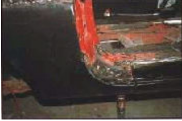
The lower wing repair section welded in to place The near side wing after spraying with primer
