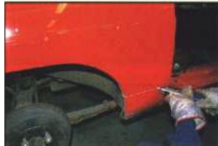
Using an air saw to start the removal process
