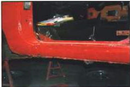
Corrosion is clearly visible along the bottom of the outer sill
