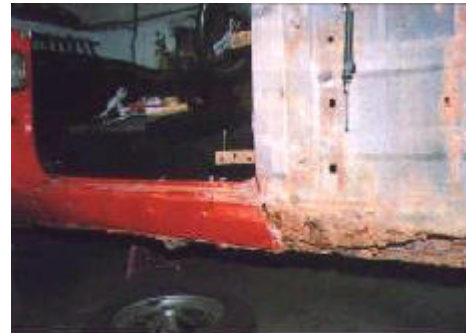
With the door and front wing removed the rust damage to the outer sill can be clearly seen on the driver's side of this MGB roadster
