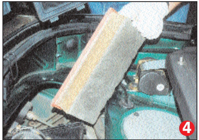
MGF air filter - note the blanket attached to this filter element base is a standard factory fit
