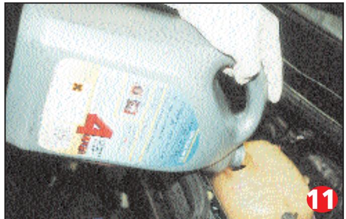
Replacing coolant with 4Life offers extra advantage of coolant colour change as warning for gasket problems
