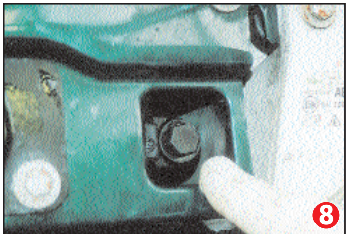
Bleed point one, at the top of the radiator
